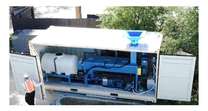
The CCM1000 is a portable batch plant that can be setup in remote locations to batch all types of concrete up to 1,000 yards per day. Structural foundation, wall panels, roof panels, lightweight geo-backfill or mine fill, roof's insulation and everything in between.
